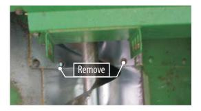
3. Remove the two carriage bolts on the left end of the trough that correspond to the two rectangular cut outs in the poly liner.
