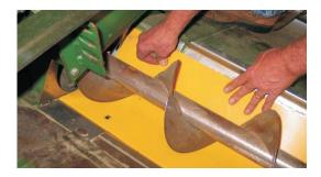
5. Loosely re-install the two carriage bolts removed in STEP 4. DO NOT TIGHTEN AT THIS TIME.
