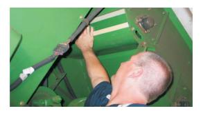
10. Position the drill template on the underside of the rear trough as Illustrated below. Firmly press the double sided tape to secure the template.
