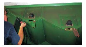
18. With all the hold down strips fastened, complete the installation by tightening 1/4" and 3/8" carriage bolts with the flange nuts provided.
