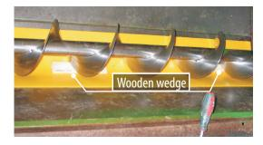
6. Use the wooden wedges supplied as required to insure that the liner is tight against the bottom of the trough.
