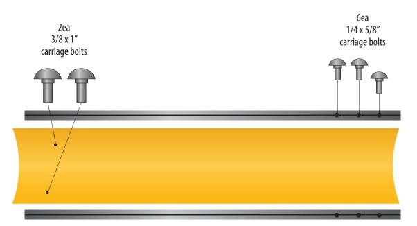
16. Loosely install the 1/4" and 3/8" carriage bolts supplied as illustrated above. DO NOT TIGHTEN AT THIS TIME.
