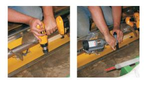
8. Install a screw or rivet in each hole before drilling the next hole. Be carefull to keep the strip straight.
