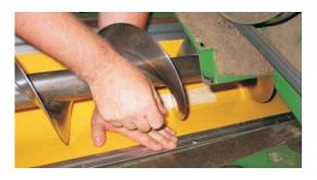
15. Secure the liner with the upper front and upper rear hold down strips.
