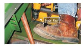
7. Install lower rear hold down strip labeled AGTJHD8825LR working left to right.
